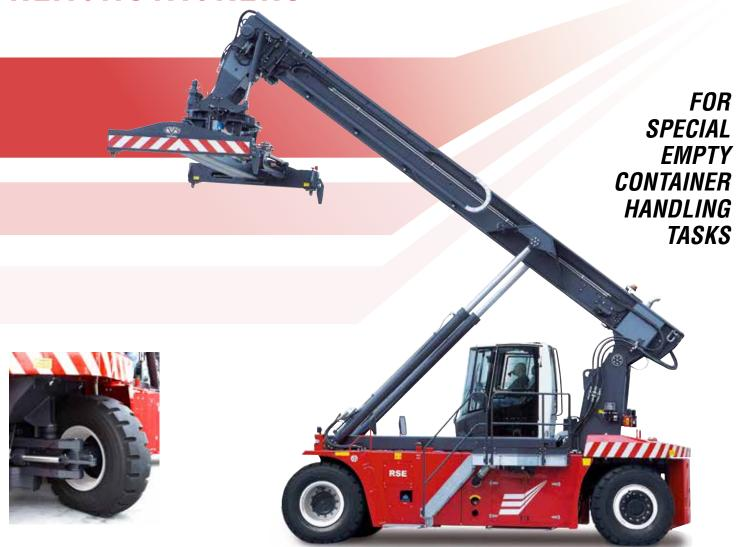
W orking in demanding applications where doorways or overhead wires must be negotiated, the CVS FERRARI RS-ECH empty reach stacker is an invaluable tool for many end users. With the ability to unload second rail from one side reaching over a first rail line or to be selective in the stack, this machine resolves otherwise problematic handling tasks and it does it with the proverbial safety and productivity of any CVS FERRARI branded equipment.
