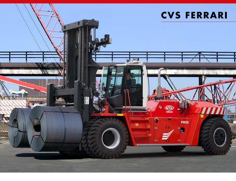
he variable displacement piston pumps and the load sensing distribution valve are electronic controlled by the CVS FERRARI landmark SIXTH SENSE system which minimizes fuel consumption and engine stalling whilst maximizing both speed and control of hoist. Lifting big loads has never been this easy.
