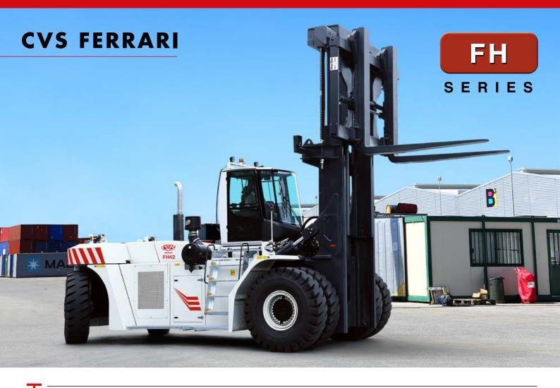
he Driver of a CVS FERRARI Heavy Forklift operates in a solid, safe spacious and comfortable environment. The ARIA cab is equipped with laminated glass, a contoured sun-deflecting front glass and is perfectly sound and temperature insulated. Its visibility and solidity are top class derived from the recessed front pillars and the FOPS upper glass. In its standard configuration it is the most complete and luxurious operator environment in the market.
