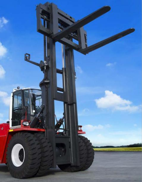
he BIG FORKLIFTS that we build at CVS FERRARI are calculated to offer the longest design life in the industry and are designed to withstand the heaviest applications and the hardest working environments. The masts of our trucks are precisely machined after they have been welded - this way ensuring perfect alignment of all its elements and minimizing play and fatigue throughout the entire structure. They are fitted with large rollers mounted on press fit spindles.
