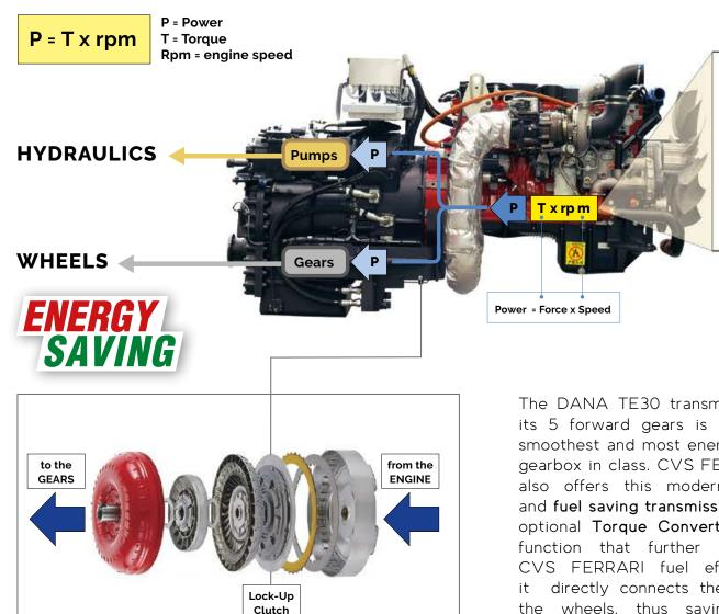
The DANA TE30 transmission, with its 5 forward gears is already the smoothest and most energy efficient gearbox in class. CVS FERRARI now also offers this modern, powerful and fuel saving transmission with the optional Torque Converter Lock-Up function that further boosts the CVS FERRARI fuel efficiency as directly connects the engine to the wheels, thus saving on the torque converter energy absorption.
