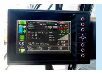
The on-board computer monitors the energy flows incoming and outgoing the battery and keeps full recording of the recycled energy.
