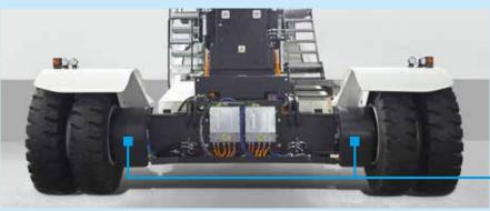
Electric motors directly mounted at the wheels eliminate the energy loss typical of conventional mechanical motion transmission. Inverters - one per each motor - provide responsive control and exceptional and progressive acceleration. The electric brake is supplemented by a wet disc brake system that renders the driver's feel the same of driving a truck with mechanical transmission.
